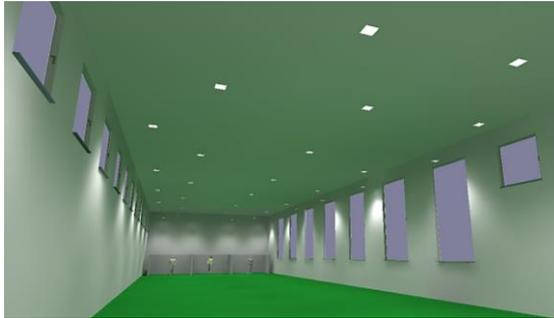
We demonstrated our own-brand LED industrial-and-sports lights. The sample featured a 90x90 degree beam with a defined cut-off. The client agreed that this gave wide and uniform illumination without creating glare when viewed from the side (ie from the batting positions).
